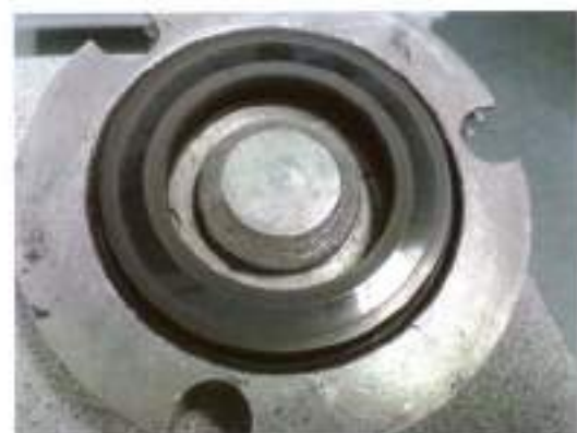
Seal face coated with CVD diamond, as it appears after 10 hours of dry running at 1500 rpm.
